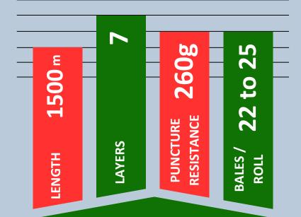
A SUPERIOR 7-LAYER COATING FILM that is manufactured in Europe. Plastitech's high-performance Amplast 7 film offers BETTER OPACITY, BETTER CLING QUALITY, AND GOOD PUNCTURE RESISTANCE. It is resistant to UV light while being airtight and rainproof.
